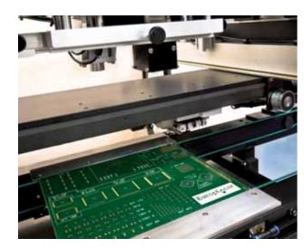
As a standard feature the vision system, developed by Speedprint, facilitates a unique 'paste on stencil' inspection feature. This enables the user to determine that there is adequate paste on the stencil before running the print cycle.
