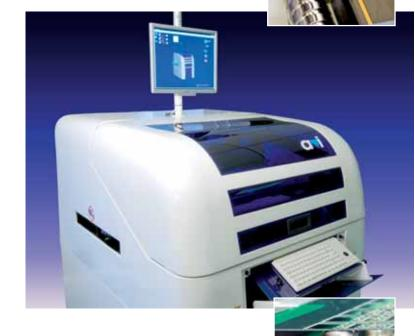
Automatic rail width adjust is standard to aid quick changeovers in a high mix manufacturing environment.
