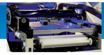
The automatic stencil loading facility enables the operator to easily switch between stencil frames at the touch of a button, thereby promoting fast changeovers and low cost of ownership.
