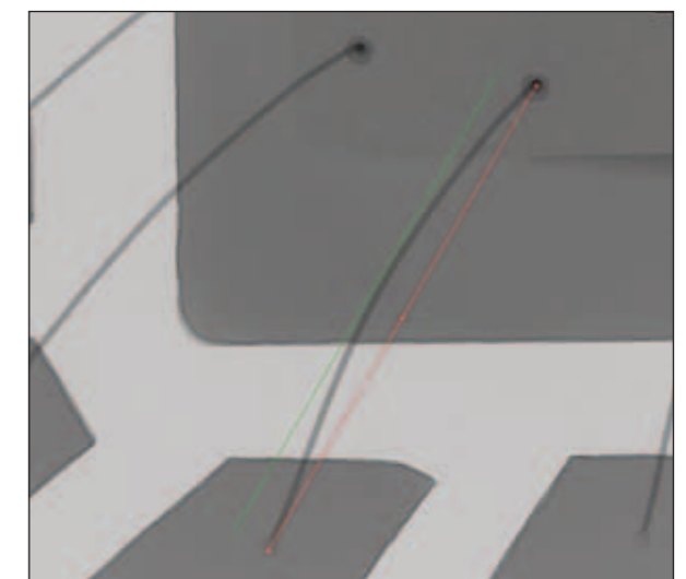
Maximum magnification - An ultra thin output window enables samples to be safely placed within 250µm distance of the focal spot providing magnification up to 6000x
