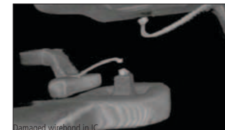
Damaged wirebond in IC
