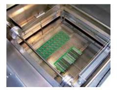
Thanks to variable temperature gradient control, a certain amount of vapour, which is adapted to the respective heat required by the modules, is automatically created. This means that the optimum temperature is ensured at all module positions so that even modules with a wide range of very different thermal requirements can be soldered. The temperature variations on the modules remain at a minimum.
