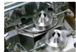
Second solder pot to process multi-up panels or two different solder alloys
