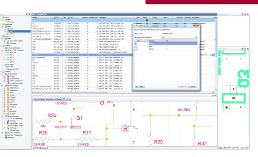
Automated DFT analysis avoids manual intervention and the generated reports show testability as opposed to accessibility through predicted DPMO and yield results. Quickly identify all components that are to be included in the AOI and AXI inspection programs.
